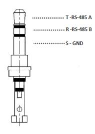
The Tally output pins on the receiver side are defined as follows.
