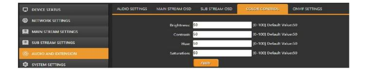
• User can adjust the brightness, contrast, hue, saturation of streaming video through the web page.
