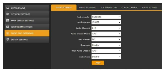
The encoder support audio embedding from external analog input. Therefore, the audio can be from SDI embedded audio or analog Line in audio. Besides, Audio Encode Mode can be ACC/ MP3/ MP2.
