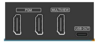
PVS0403U has 4 output interfaces. They are default as 2PGM Out, Multiview Out and USB Out. All the 3 outputs also can be defined as an AUX OUT from SDI1, SDI2, HDMI3, HDMI4, PVW, PGM, Clean PGM, Color Bar and Multiview out.
