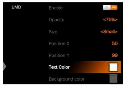
The UMD string content for 2SDI and 2HDMI inputs can be set from menu. User can rename the UMD content for each window by using a virtual keyboard and rotary button. It supports input max 10 characters for the UMD content. Below image as an example, rename the SDI1 to CAM1.
