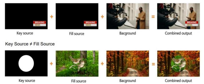
Luma keys provide a way to composite a Text clip over a background clip based on the luminance levels in the video. Turn on the Luma Key, a color from the key source will be removed, revealing another background image behind it.
