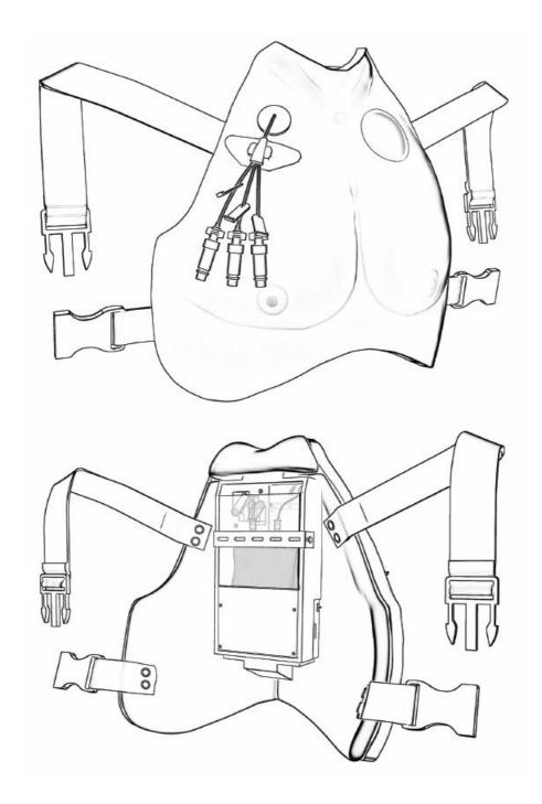
Welcome to your Avline five heart sound locations can be controlled through the Avkin App antimicrobial blood for blood draw and flushing Standardized patients are cued through a light vibra- tion on the shoulder to provide a patient response when pressure is applied around the central line or to the port-a-cath. Learners receive real time feedback about their care
