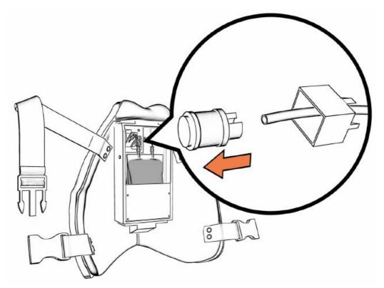
4. Pull out silicone insert from port-a-cath and wipe down both the plastic and silicone components with paper towel. Snap the silicone back into place when complete.
