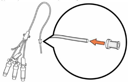
2. To reinstall the central line into chest, remove connector on central line, poke central line through hole in chest and align with hole in chestplate assembly to feed through to back of the device.
