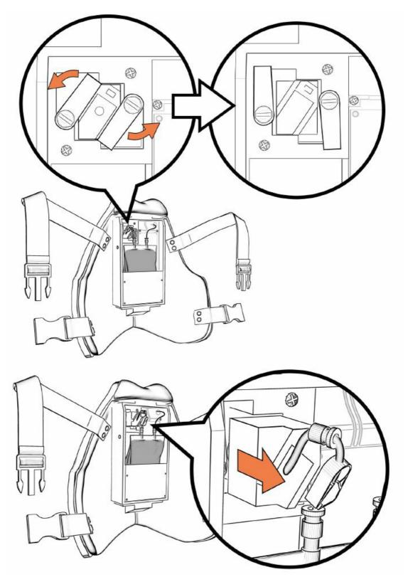
3. Remove port-a-cath from device by sliding out port-a-cath housing and disconnecting tubing connection.
