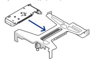
8. Push the expansion card riser back into place and close the expansion card latch.
