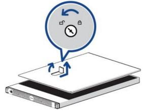
Inside the recorder, be cautious of cables from the RAIDcontroller (PERC) that may obstruct access to the expansion cardriser. Install the analytics kit without disconnecting the cable,taking care not to pull or strain the PERC cable duringinstallation.
