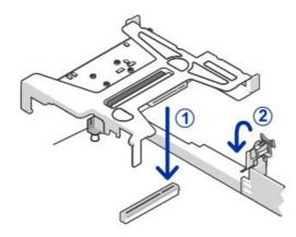
9. Align the slot on the air shroud with the standoff on therecorder. Then lower the air shroud until it is firmly seated inplace.
