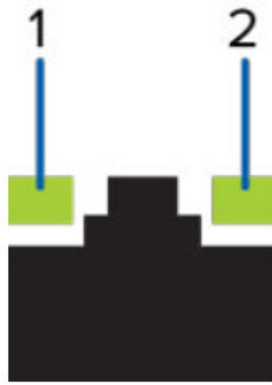
Figure 7: (1) Link LED. (2) Connection activity LED.
