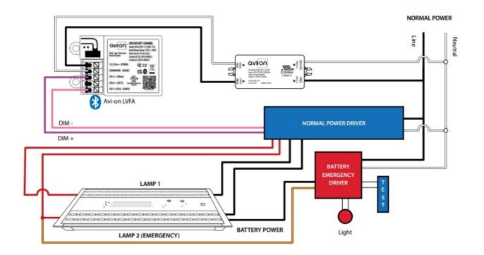
Connect the Normal Power Driver AC, Battery Emergency Driver AC and 110-277v -12VDC power adaptor to the Normal Power AC. Connect the low voltage outputs from the power supply to the Avi-on LVAC power Plus and Minus Inputs. Connect the LVFA Dim+ and Dim- wires to the driver as normal.
