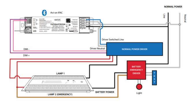
Connect the Battery Emergency Driver AC and Avi-on IFAC AC inputs to line and neutral of the normal power circuit. Connect the Normal Power Driver AC inputs to the AC driver outputs of the IFAC. Connect the IFAC Dim+ and Dim- wires to the driver as normal.
