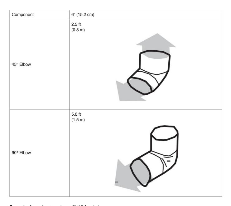
Example of an exhaust system – 6" (15.2 cm) pipe
