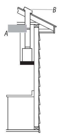
A. Duct of 6" (15.2 cm) in diameter to discharge through the roof B. Discharge exit through roof **Evacuation through the wall**
