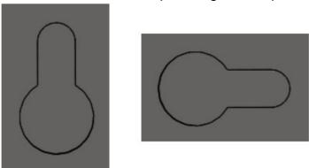
Key on back of codec should be point upwards or sideways in mounted position.
