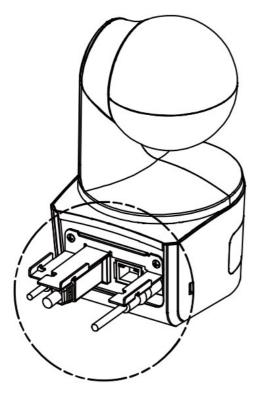
3. Use 3 cable ties in the package to secure the cables and cable fixing plate.
