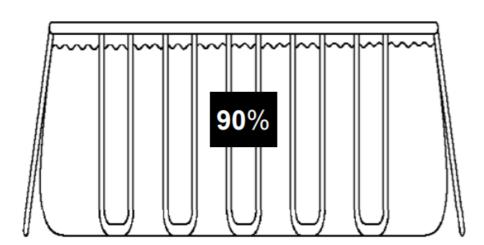
1. Make sure the drain fitting is plugged securely and the cap is in place. Start filling the pool with water. After about 1-inch of water is on the bottom, stop filling and smooth wrinkles out of the bottom of the pool. Pull the outer wall out from the top edge, all around the bottom of the pool, so that it fills evenly.
