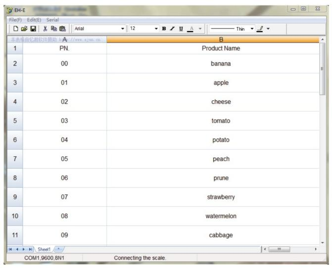
2. Connect the scale with the computer via RS232 port, then power on the scale. Normally, the scale will be automatically connected to the computer and shows"This scale is connected". If not click the "Serial" menu on the software to set the baud rate to 9600 and Data to 8N1, then confirm by clicking "open port".
