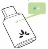
3. Non-1st time use, manually enter C81 into pairing mode: Press & Hold MB until LED flashes BLUE & WHITE
