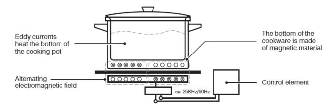
The cookware must be magnetic. Before switching on the appliance always place the magnetic cookware centered onto the cooking field.
