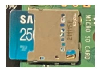
Pro Tip: Use some tape on top of the SD card and metal slot in order to prevent it from sliding out over time.
