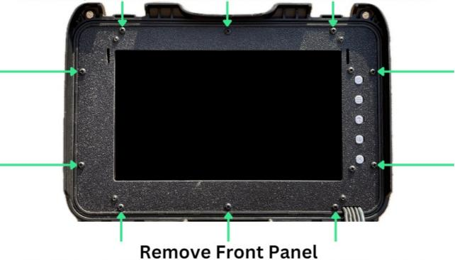
Pro Tip: Place a cloth to protect the front panel while being serviced.
