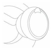
2. Vertically insert the bottle into the bottle supporter (#1) on the top of the machine. The bottle supporter has a
