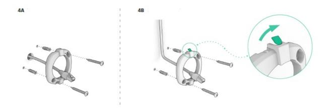
Attaching the camera and connecting the ethernet cable
