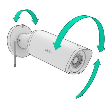
When the correct position is obtained, firmly tighten the screws (3-4Nm) to lock the position.
