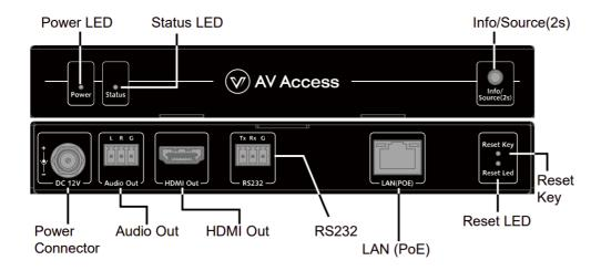
Info/Source (2s) Key: Short press to display/stop displaying information of encoder and decoder on screen; press and hold for 2 seconds to link the decoder to another encoder.
