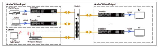
3. Configure the wireless router properly, then connect your iPad to the Wi-Fi network. Launch VDirector on iPad, it will start searching for online devices, and the following main screen will appear:
