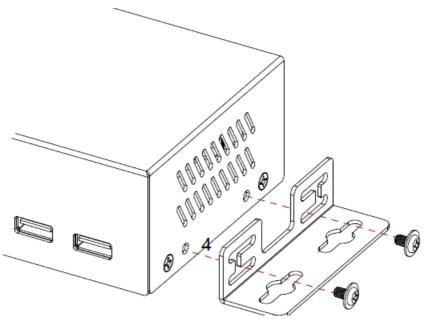
2. Attach the brackets to the surface you want to hold the unit against using the screws (provided by others).
