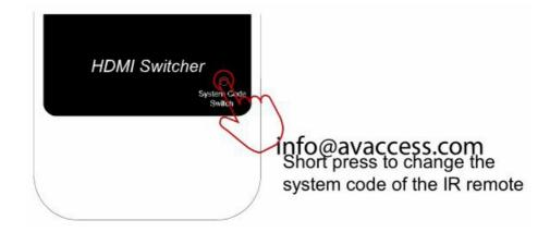
The IR Remote provided with the switcher is shipped in "00" IR system code. In the event that Remote's IR signal interferes with IR devices, e.g., TV, DVD player, the Remote can be switched to "4E" code by short pressing the System Code Switch on the Remote panel.
