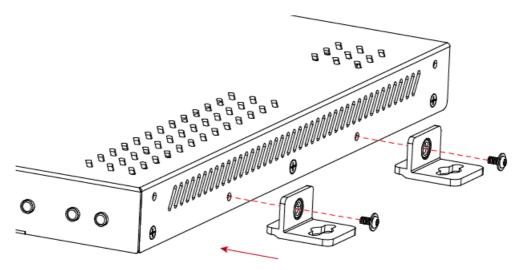
2. Install the brackets onto the position as desired using the screws (not included).
