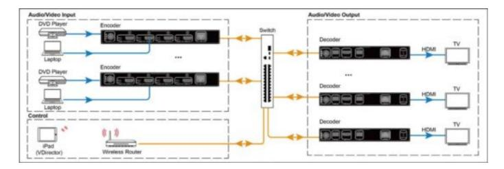
3. Configure the wireless router properly, and then connect your iPad to the Wi-Fi network. Launch VDirector on iPad, it will start searching for online devices, and the following main screen will appear:
