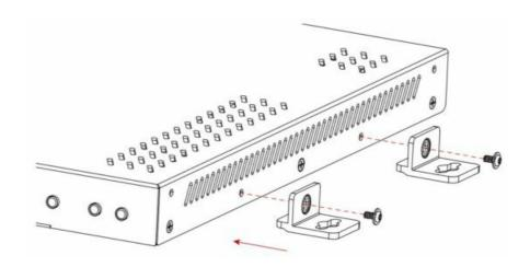
2. Install the brackets onto the position as desired using the screws (not included).
