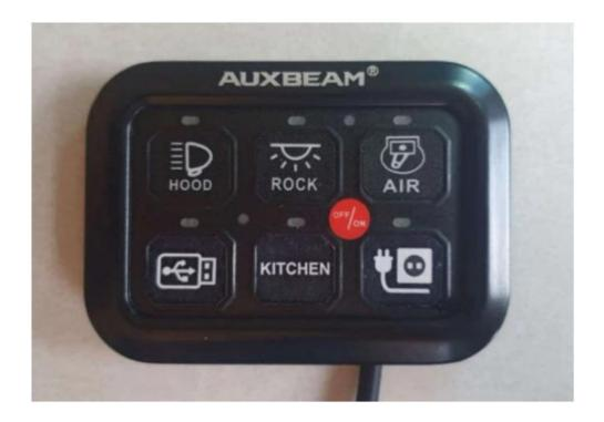
When the switch panel is illuminated, the custom labels are a little brighter than the Auxbeam labels. You may like the extra brightness better, but if you'd like them to be the same brightness as the Auxbeam labels you can use a double layer of the label stock too so less light passes through the custom label.
