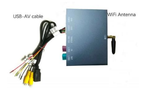
The CarPlay interface decoder box should be installed in an appropriate space near or on the OEM head unit.
