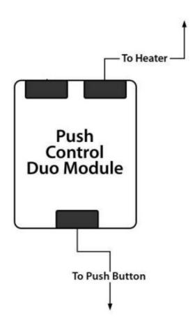
After connecting the module to the heater, successful connection with the heater is indicated by LED flash RED/Green. When it stops, it indicates that AUTOTERM Push Control has successfully connected with the heater. The Module must be mounted in a secured and dry environment as the module by itself does not have any ingress protection!
