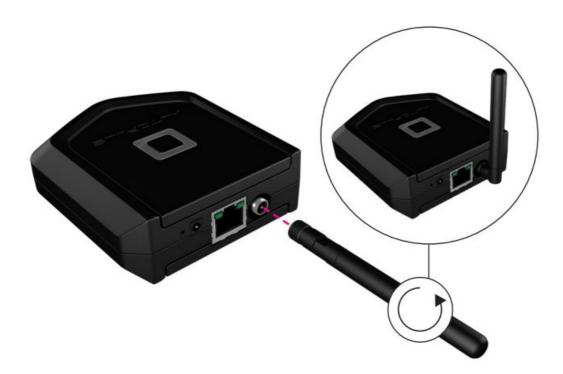
1. Connect the antenna to the back of the AutoPlus and tighten by turning clockwise. Position the antenna to a straight up position.
