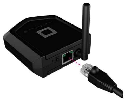
2. Plug the Ethernet cord into your router and connect the other end to the back of the AutoPlus.
