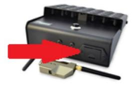
The receiver will confirm the units are paired when the LNK light is illuminated GREEN. The receiver will confirm data is being transmitted when the OPR light is flashing RED.
