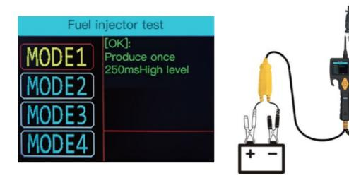
The probe outputs different pulse signals to the injector, and check the injector spraying status. This function can help diagnose injector conditions. It can work with any fuel pressure tester.
