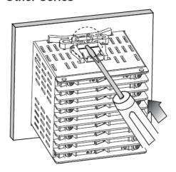
• Insert product into a panel, fasten bracket by pushing with tools as shown above.
