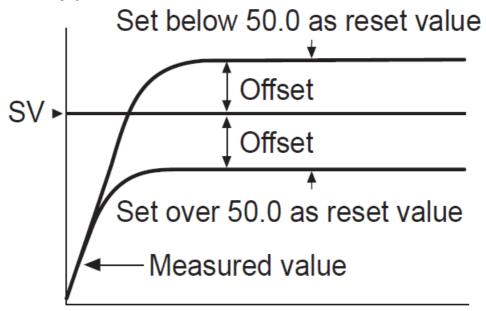
When selecting P/PD control mode, certain temperature difference exists even after PV reaches stable status because heater's rising and falling time is inconsistent due to thermal characteristics of controlled objects, such as
