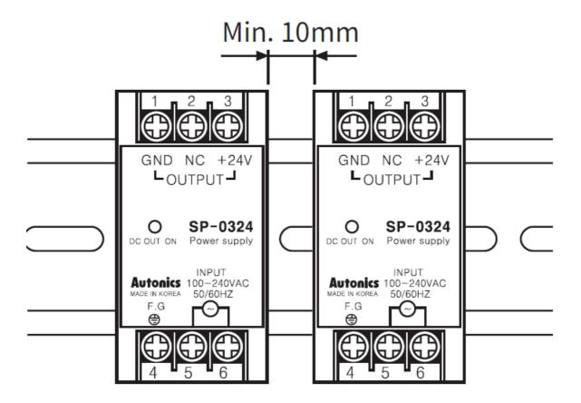
When installing multiple SMPSs, please keep space at least 10mm between SMPSs for heat radiation.
