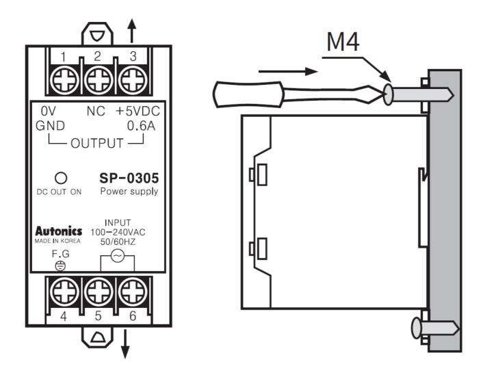
If there is no rail, it is able to mount by screwing a bolt at the hook on the body as following figure.
