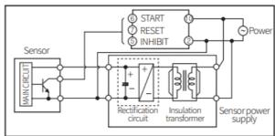
In order to avoid leakage current flowing, connect resistance and condenser like below. Otherwise, it may cause malfunction.
