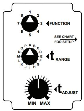
**Setting Function:** To set the function, first select one of the eight TRM-8 Series functions from the Select Function Chart located on the side of the relay. Position the eight-position rotary switch to the number that corresponds to the desired function.
