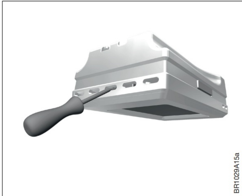
Fig. 2 Removing the front cover
