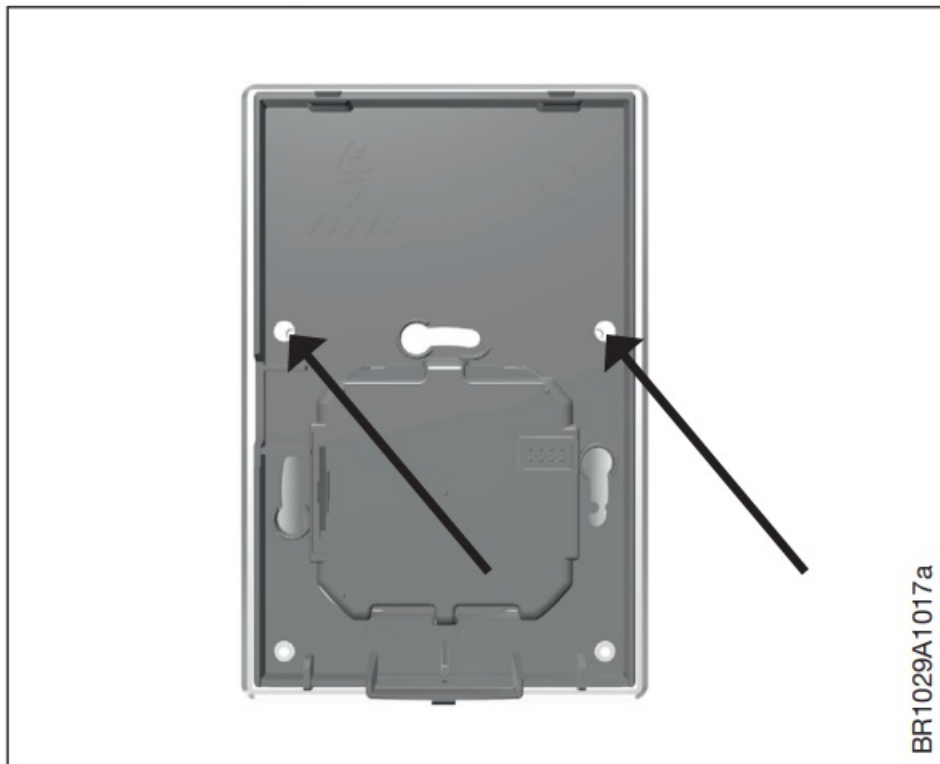
Fig. 3 Removing the back cover
