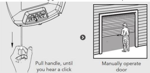
**CAUTION:** When the opener is manually disengaged, the door is no longer locked. To lock the door manually, re-engage the opener after the door is closed.
