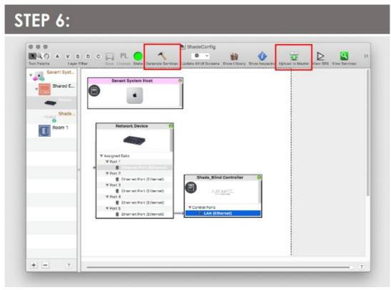
6. Click the "Generate Services" button again, then "Upload to Master" to push the configuration to the Savant Host.
