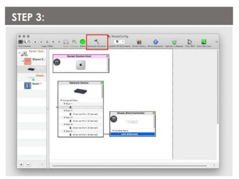
3. Make a connection between the "LAN (Ethernet)" port on the Shade Controller profile and the "Ethernet Port (Ethernet)" port on a Network Switch profile. Then click the "Generate Services" button.
