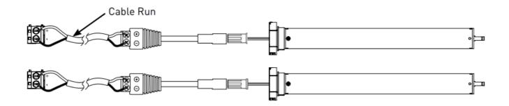
This connection may only be used when wiring 28mm & 25mm motors to the distribution panel, as these motors do not exceed the 1.33 A current limit per channel.
