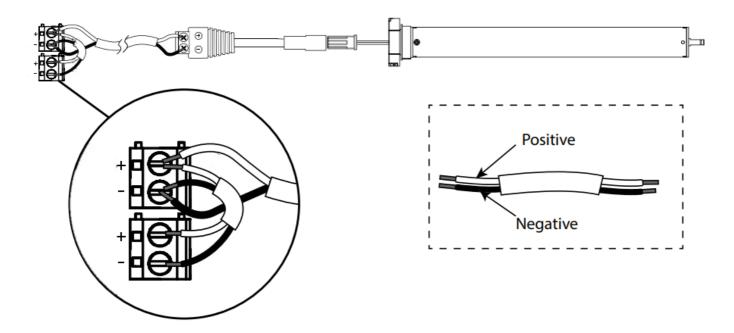
Due to the 1.33A limit per channel, the working current can be doubled to 2.66A with parallel configuration, as shown above, allowing a connection of 45mm and 35mm motors.
