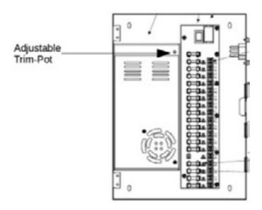
If motors powered by the DC Power Distribution Panel are to be used with the Automate Pulse 2 Hub and Application, the output voltage of the Distribution Panel MUST be adjusted to allow for proper communication between the Hub and Motor. Output Voltage (11.4VDC to 15VDC) of the DC Power Distribution Panel can be adjusted via the Trim-Pot located on the converter within the Distribution Panel.
