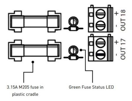
In order to replace the fuse, carefully pry the fuse out of the plastic cradle using a small tool (such as a small screwdriver or pen). To replace, gently press the new fuse into the cradle. To test LED, apply power to the distribution panel, and observe whether the channel LED is glowing.
