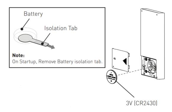
**STEP 3**Slide up to lock the battery door
