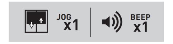
Within 4 seconds hold the stop button on the remote for 3 seconds. The motor will respond with Jog and Beep.
