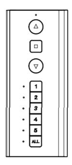
Select a single or multiple channels by toggling channels as required. Note the corresponding LED next to each channel.
