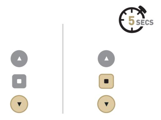
Move shade to desired bottom limit by pressing the down arrow repeatedly. Then press and hold down & stop together for 5 sec to save limit. Tap the arrow several times or hold down if needed; press arrow to stop.
