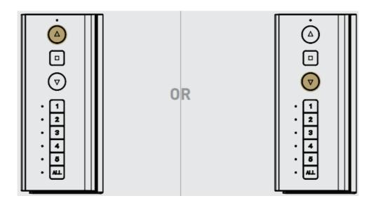
While the channel is displayed press up or down to move shade accordingly.
