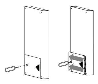
**STEP 2**Install CR2450 Battery with positive (+) side facing up.
