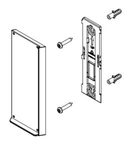
Use supplied fasteners and anchors to attach the base to wall.
