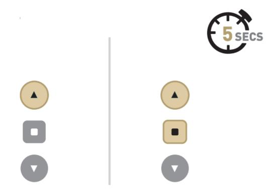
Move shade to desired top limit by pressing the up arrow repeatedly. Then press and hold up & stop together for 5 sec to save limit. Tap the arrow several times or hold down if needed; press arrow to stop.
