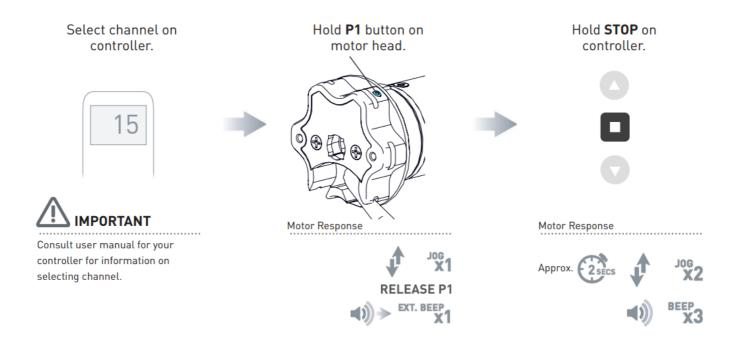
Motor is now in step mode and ready for setting limits 6.1.2 Check motor direction
