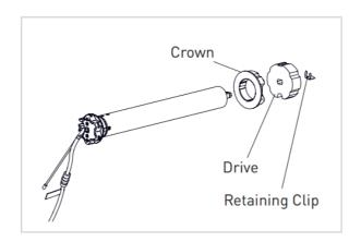
Step 4. Slide Motor into the tube. Insert by aligning the key-way in the crown and drive the wheel into the tube.
