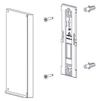
Use supplied fasteners and anchors to attach the base to wall.
