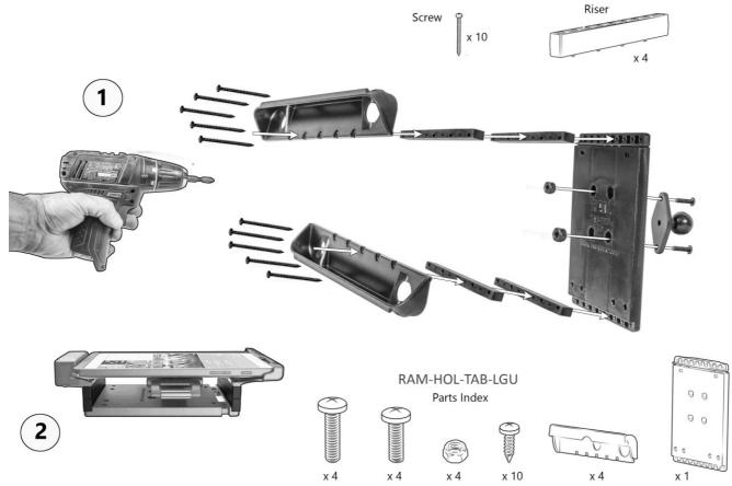
Tablet Cradle with risers installed so the tablet will fit properly in the RAM Mount Cradle.
