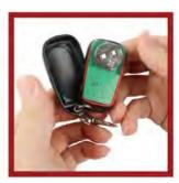
Before using the Remote Control Switch, please pull out the insulation sheet on the battery. If you want to replace the battery, use a fingernail or a tool along the edge of the remote control to pry the top cover open. (As shown above.) A gentle push en take out the battery. After replacement, close the cover and you'll hear a "elide' sound as it tight close.
