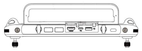
Fig 4-16 Custom Keys C1 and C2
