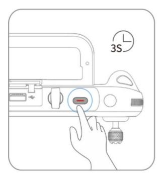
Fig 4-6 Turning the Remote Controller On
