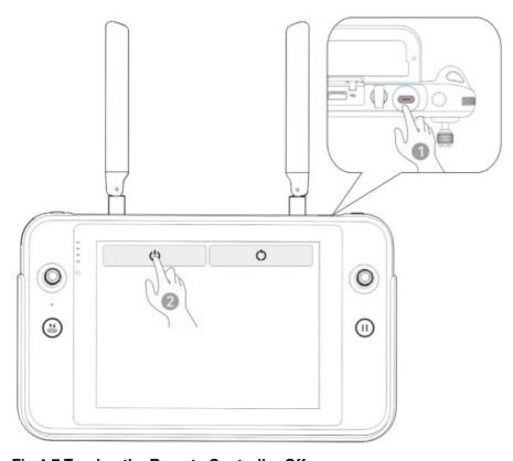
Fig 4-7 Turning the Remote Controller Off
