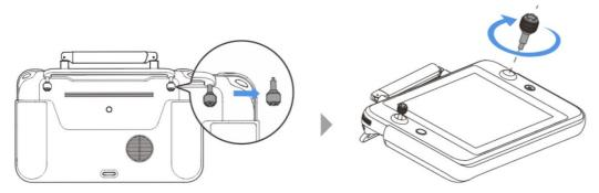
Fig 4-5 Installing command sticks
