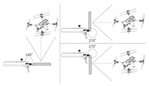
Fig4-10 Extend the antenna
