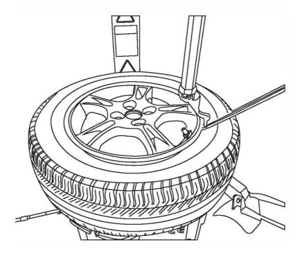
CAUTION This starting position must be observed during the whole dismounting process Dismounting the sensor
