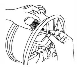
Remove the cap, screw nut, and washer from the valve stem, and then remove the sensor assembly from the rim
