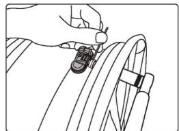
Mounting the tire Place the tire on the rim, make sure that the valve faces the separation head at an angle of 180 °. Mount the tire over the rim.
