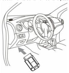
• Insert the MaxiVCI V150 into the vehicle's DLC, which is generally located under the vehicle dashboard.
