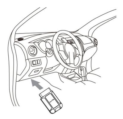
• Insert the MaxiVCI V150 into the vehicle's DLC, which is generally located under the vehicle dashboard.
