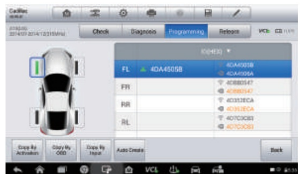
Program Success (MX-sensor ID is copied from the activated sensor ID)
