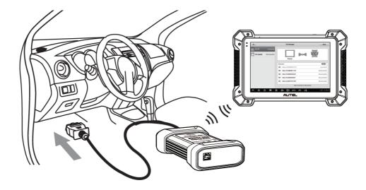
Pair up the MaxilM IM608 Pro II tablet with the VCI device via Bluetooth to establish a communication link with the
