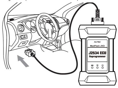
Connect the VCI with the vehicle's DLC, which is generally located under the vehicle dash.
