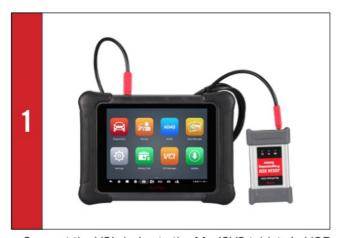
Connect the VCI device to the MaxiSYS tablet via USB
