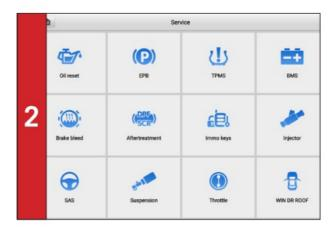
Designed to provide quick access to the vehicle systems for various service and maintenance tasks. Comprehensive service functions, including Oil Reset, EPB, SAS, OPF, TPMS, and BMS.
