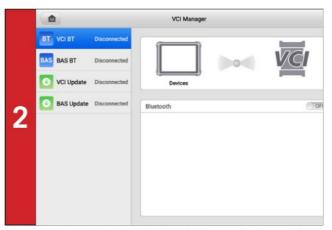
Your tablet will automatically start scanning for available VCI devices. Found devices are listed on the right side of the screen.
