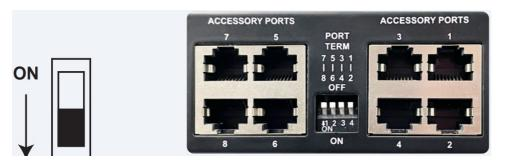
2. Terminate the LAST RS485 accessory on the port cable run.
